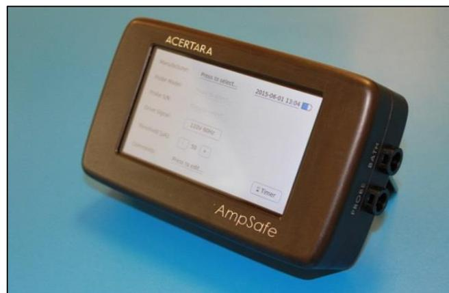
**TEE Electrical Leakage Device - AmpSafe**
